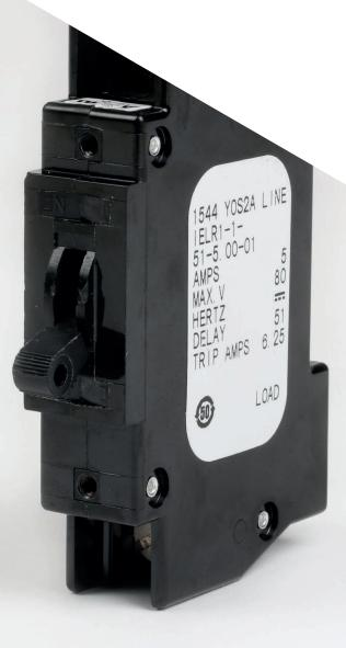
Hydraulic Magnetic Circuit Breakers do not employ the use of any thermal element to carry out the objective of current monitoring. Therefore, allowing the Circuit Breakers to operate in parameters not affected by adverse environmental conditions.
